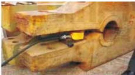
Only the low height HHYG cylinders are suitable for use in this confined space.
