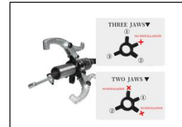
3. The jaws have four different settings. Each can be for both inside and outside pulling. Determine whether to use the upper or lower holes in the Jaws and which way the jaws should be turned.
