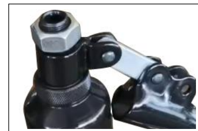
4. Expose the oil filling port
