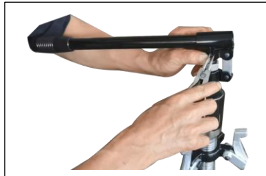
1. Use circlip pliers to remove the circlip
