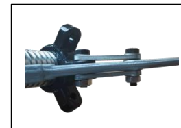
4. Assemble each of the three Jaws onto the Puller Sleeve using two Connector Plates and two Bolt Sets as shown.
